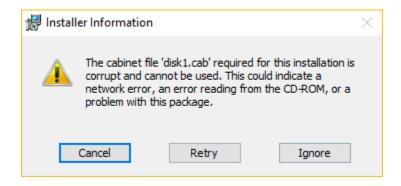
If this error occurs, simply copy the "msi" files from the USB drive to a temporary folder on the PC and re-execute.
