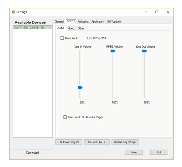
To modify audio settings, modify the settings to desired values and press **Save** to send the settings to the ChyTV device. Select Restart ChyTV App to apply the settings.
