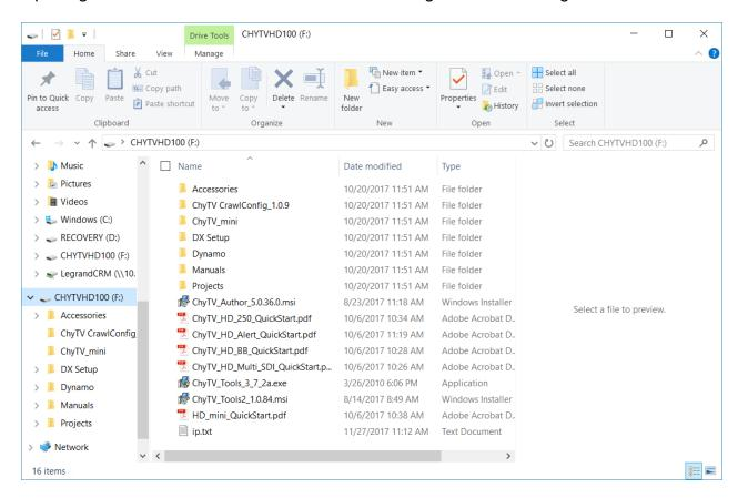
The same exact thumb drive image is used for all of our products. The CHYTVHD100 volume label is actually used a 'precaution' for using the thumb drive for configuration updates. The IP.TXT file on the thumb drive can be modified for a variety of commands to the device, most commonly is to change the networking parameters. When a thumb drive is inserted in the device, it first checks for the CHYTVHD100 volume name, otherwise no action is taken.
